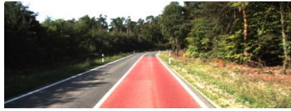
Fig. 15 Highlighting lane in unwarped image
